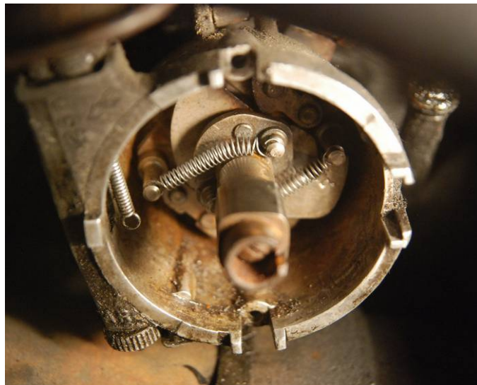
Fig. 1. Advance mechanism locked using springs
